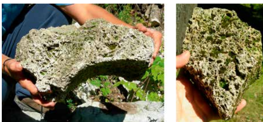
Fig. 6. Pieces of worked tufa stone found in the rubble: A – cut in the form of an arch, and B – wedge-shaped (photo: author, 2006.)
